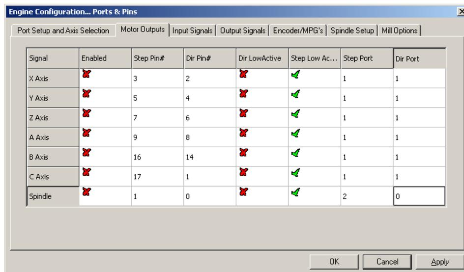
FIGURE 11 AXIS SETUP
