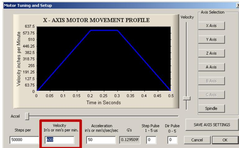
FIGURE 35 VELOCITY IN MOTOR TUNING
