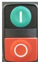
FIGURE 195 CYCLE START AND FEED HOLD BUTTONS
