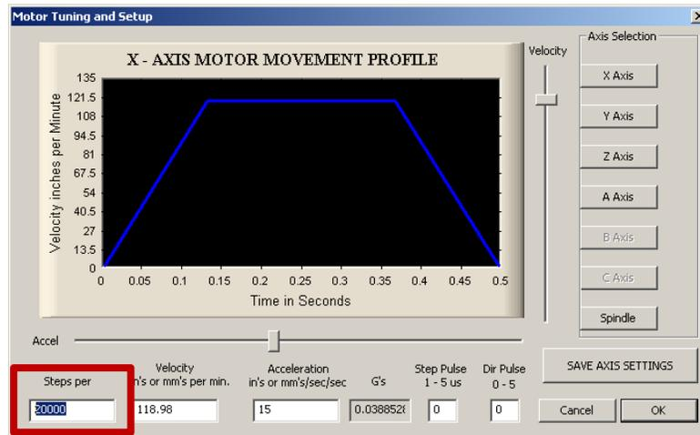
FIGURE 32 STEPS PER IN MOTOR TUNING
