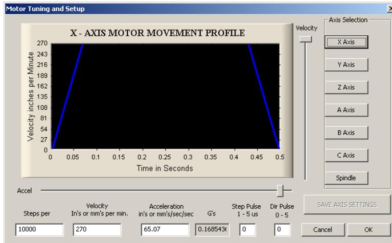
FIGURE 31 MOTOR TUNING AND SETUP
