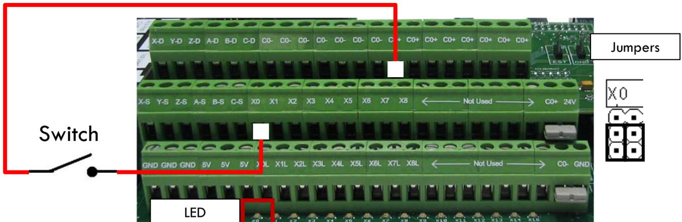
FIGURE 46 STANDARD 24V INPUT
