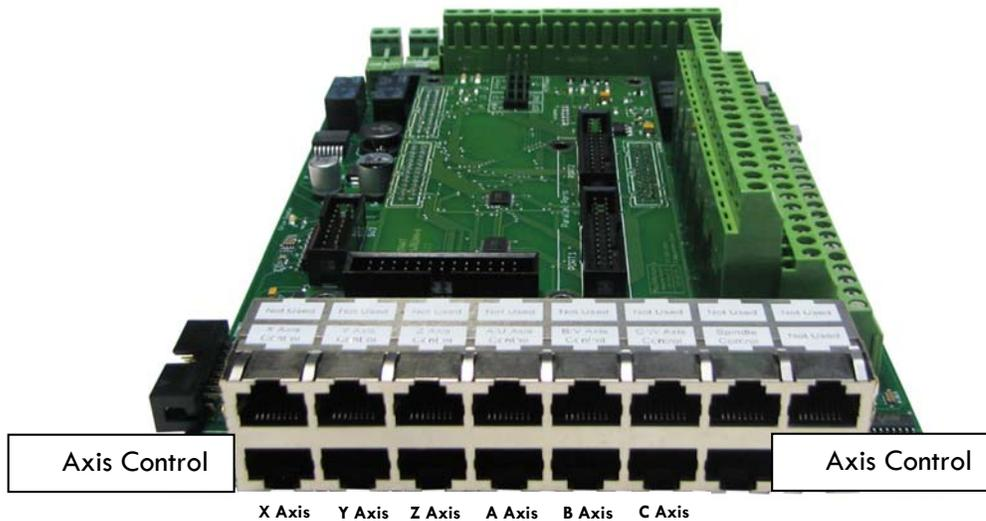
FIGURE 10 DIFFERENTIAL STEP AND DIRECTION MOD JACKS
