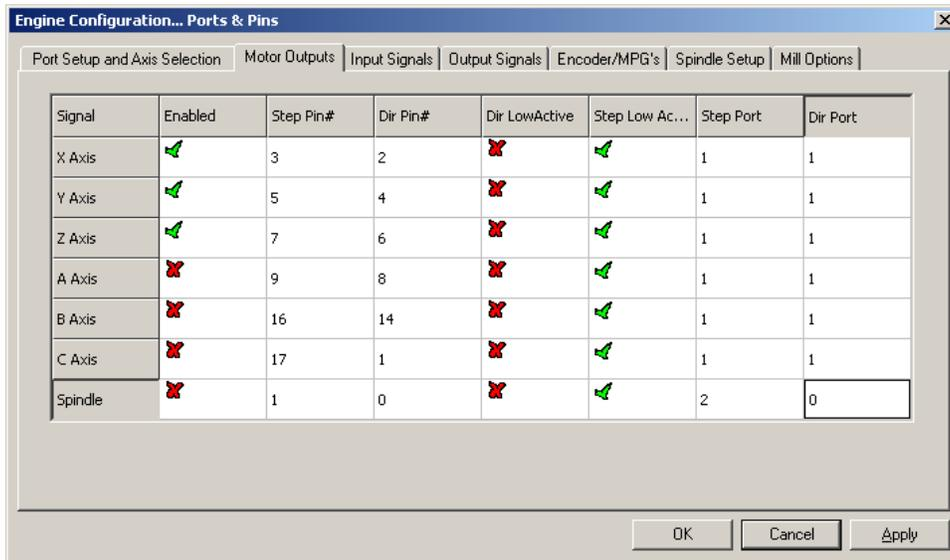
FIGURE 12 X, Y, AND Z AXES ENABLED
