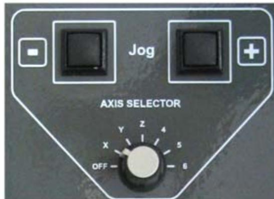
FIGURE 15 JOG BUTTONS AND AXIS SELECTOR
