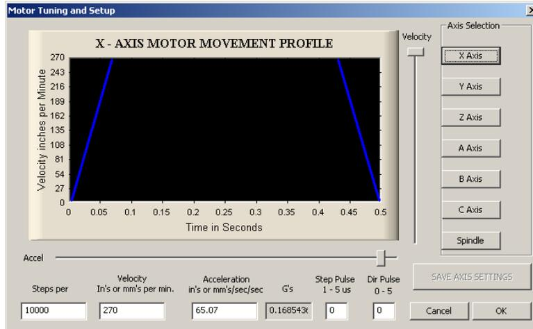
FIGURE 13 MOTOR TUNING AND SETUP
